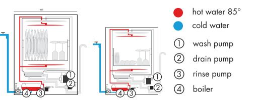
The double-wall structure, the thermal-acoustic insulation of the wash chamber and the hydraulic circuit (optimised to prevent cavitation) make Smeg Foodservice dishwashers extremely silent in all working conditions.
