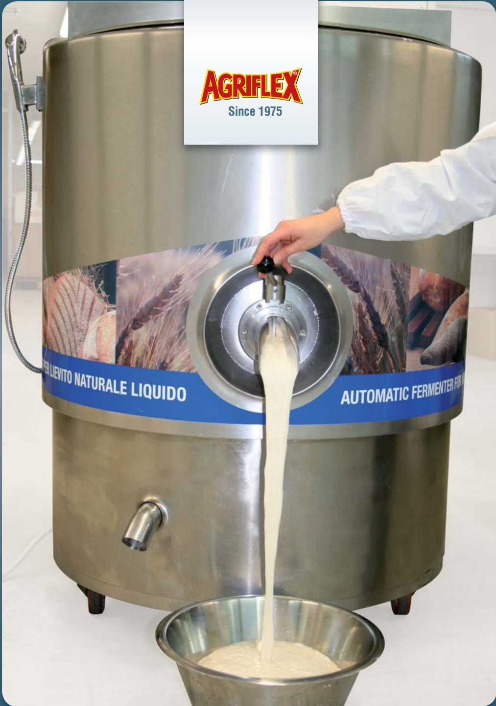
Automatic fermenter for natural liquid yeast
